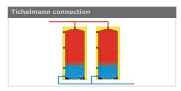
From boiler outputs of 100 kW this system is increasingly used, as the flow and return connections (DN40) at a flow speed of approx. 1 m/s have a flow volume of 4.5 m³/h, which corresponds to an output of approx. 100 kW. If there are several layered tanks the volume flow is divided evenly and boilers with an output of over 100kW can be connected to the system and used.
