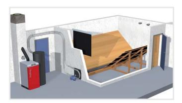
The Froling suction screw system is the ideal solution for large rectangular rooms with frontend removal. The deep and horizontal position of the discharge screw means the space in the room is used optimally and complete emptying of the store is guaranteed. Combined with a suction system from Froling it also enables flexible boiler setup.
