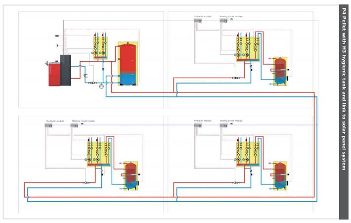
The Lambdatronic can control four layered tanks and four feeder pumps.. A maximum of four buildings can be controlled in total. There is also the option of connecting a solar system, and the position in the system is flexible (building 1, building 2 ...).
