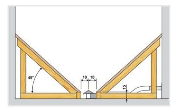
The suction probes must be equidistant and must be fixed to the floor.
