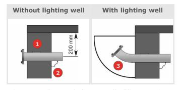
When installing a lighting well, filler couplings with 45° bends (3) are used, so the filling hose can be connected in a straight line.
