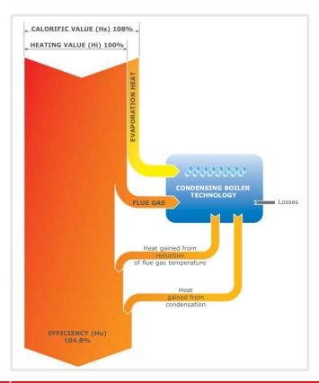
The heating value (Hi) defines the amount of heat, which is released during combustion. The water that is produced is contained as steam in the flue gas. The calorific value (Hs) defines the amount of heat that is released during combustion including the evaporation heat.
