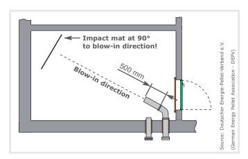
Solutions with an angled inlet nozzle must be built with a settling section of at least 50 cm after the bend and the impact mat must be opposite, perpendicular to the blow-in direction.
