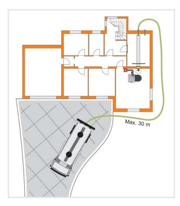
There is a limit to the filler hose length that can be used. The store should be located not more than 30 metres away from where the silo lorry will be pumping.
