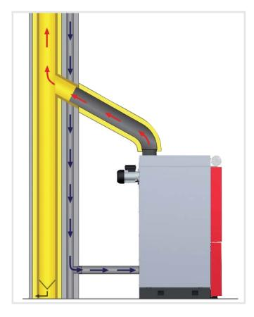
Energy-saving houses have a closed building shell. In traditional heating spaces there can be uncontrolled heat loss from the necessary ventilation openings. This is avoided with room airindependent heating boilers because of the direct air connection. The combustion air that is fed in is also heated with an integrated pre-heating system, increasing the efficiency of the system.
