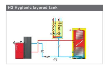
The Froling H2 hygienic layered tank offers this connection option, for hygienic domestic hot water preparation using the flow principle.
