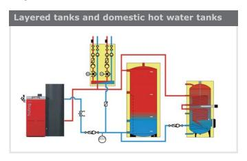
If, for space reasons, it is not possible to combine a layered tank and domestic hot water tank (see diagram above), Froling also offers layered tanks with integrated element for hygienic domestic hot water preparation.
