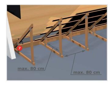
Depending on the static load (e.g. excessive distances) intermediate supports may be necessary.
