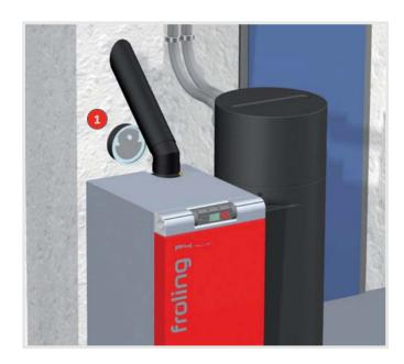
The optimum position for installation of a **draught limiter (1)** is in the chimney directly below the mouth of the flue gas line.
