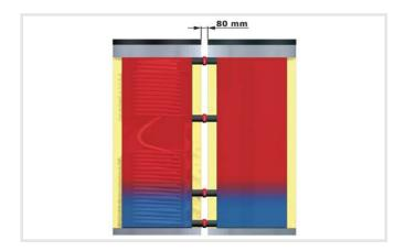
The layered tanks can either be set up in a row or at an angle. In this case the connection couplings are fitted to the layered tank in the middle at an angle of  $90^{\circ}$ .
