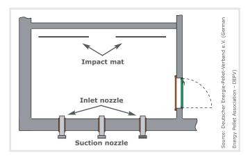
If it is not possible to install the filler couplings on the narrow side of a rectangular room, several inlet nozzles can be positioned with a separation of approx. 1.5 m. An impact mat should be fitted opposite every inlet nozzle. The main disadvantage of this solution is that the filling process must be interrupted to reconnect the filler line.
