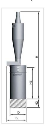
The PST pellet deduster is fitted in any position in the return air line of the pellet suction system. The suction cyclone design means that the dust particles are separated from the return air and deposited internally. The container is convenient to remove and transport to the emptying point. The system can be retrofitted at any time and it is maintenance-free except for emptying the container.
