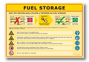
The fuel store sticker supplied indicates the hazards in the store and explains the necessary steps for filling. The sticker must be applied in a clearly visible position in the area of the store.
